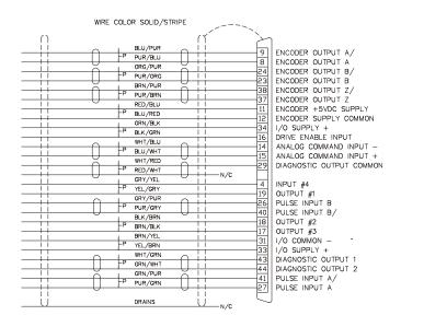
N/C = TRIM ALL WRES EVEN WITH THE CABLE JACKET  $\label{eq:result} \bigcup_{l=P} \mbox{FOIL SHIELD}$
